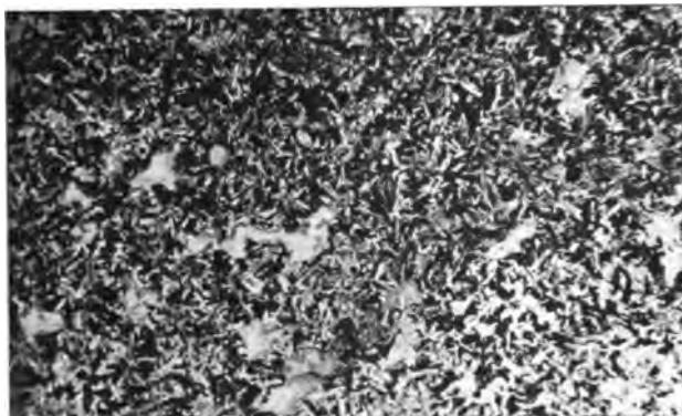
A. PEWABIC LODGE, QUINCY MINE. PHOTOMICROGRAPH X 10. THIS SECTION SHOWS A PSEUDO-AMYGDALOIDAL PORTION OF THE LODGE FROM NEAR THE FOOTWALL. THE LARGE TRANSPARENT PATCHES ARE SECONDARY CHLORITE. THEY HAVE NOT THE CHARACTER OF TRUE AMYGDULES.
